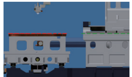
The height of the working table surface and Y axis guideways are the same which reduces the Abbe error.
